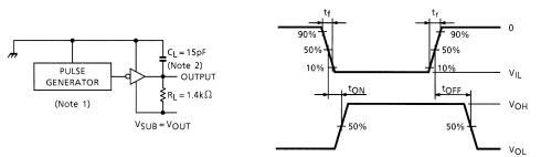
Note 1: Pulse width 50  $\mu$ s, Duty Cycle 10% Output Impedance 50  $\Omega$ , t<sub>r</sub> ≤ 10 ns, t<sub>f</sub> ≤ 5 ns Note 2: C<sub>L</sub> includes probe and jig capacitance.
